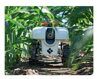
Autonomous robots fitted with cameras and sensors can be deployed in fields to monitor crops for any sign of disease or pest infestation
