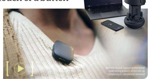
The Sound Capsule system integrates eight Nordic SoCs—including four flagship <u>nRF5340</u> SoCs and four nRF52833 SoCs. The nRF5340's application processor can supervize the demanding task of encoding and decoding the audio stream, while the network processor takes care of communication.
